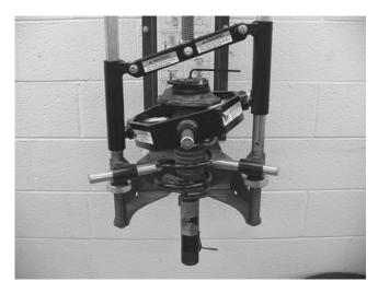
**STEP 6:** Disassemble strut-spring assembly. The following parts will be reused in assembly; top mount, bearing, spring seat and boot.
