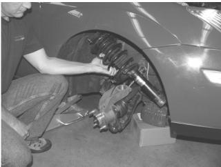
!!! Warning: Spring is under extreme compression. To avoid personal injury use a suitable spring compressor!!!
