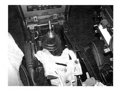
Remove rubber dust boot by pulling it up and off the shifter
