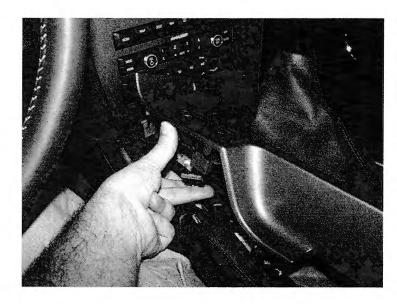
Carefully set the center trim piece on the passenger seat being careful not to damage any wiring in the process
