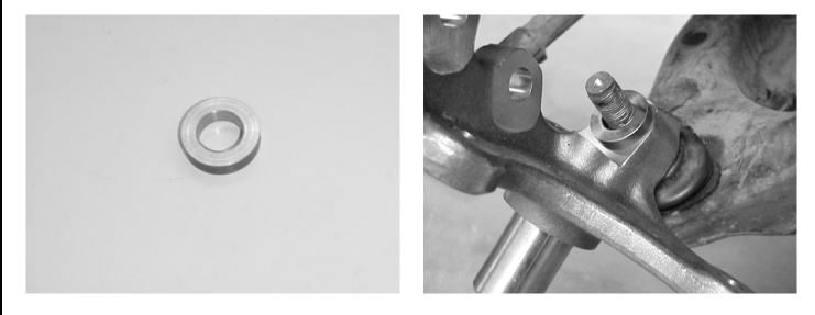
**STEP 21:** Install the original ball joint nut on the stud. Do not tighten at this time.
