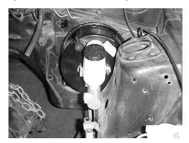
**STEP 5:** Reconnect the wiring harness plug to the master cylinder float switch.
