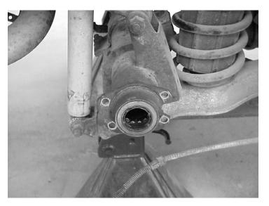
**STEP 13:** Reusing the backing plate bolts, install the caliper to axle adapters (item 38 and 39). Torque bolts to 45-50 ft./lbs. Axle adapters are marked LH and RH. The RH is shown below.
